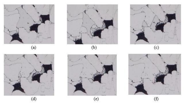
**Fig. 4:** Dissolved bubble blocked from protruding into geometry. The images are ordered chronologically from (**a**) to (**f**)
