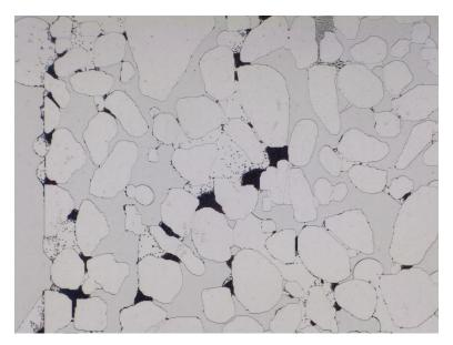
Fig. 3: Clogged pores successfully blocking gas phase from expanding
