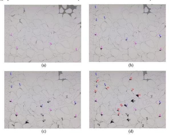
**Fig. 1:** Accumulative clogging through developing pathways. (a) was acquired at 10:46, (b) was acquired at 10:51, (c) was acquired at 10:53, and (d) was acquired at 10:54. The colors indicate when each clogging event occurred. The colours of purple, blue, black, and red indicate clogging developments for images (a) through (d)chronologically, respectively.
