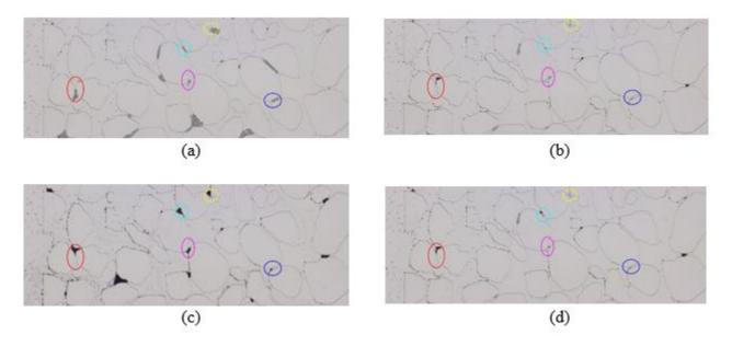
**Fig. 2:** Residual gas bubbles blocking colloid attachment and pore clogging prior to dissolving. Images (**a**) through (**d**) are ordered chronologically, with (**a**) being acquired first, and (**d**) being acquired last
