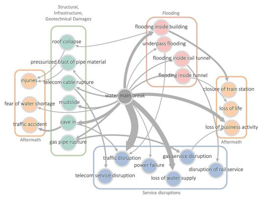
Fig. 3: Sequence of damages and disruptions from watermain breaks
