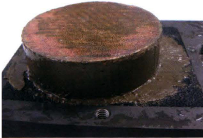
Figure 2.3. UWA small-scale direct shear box (after White et al. 2012)
