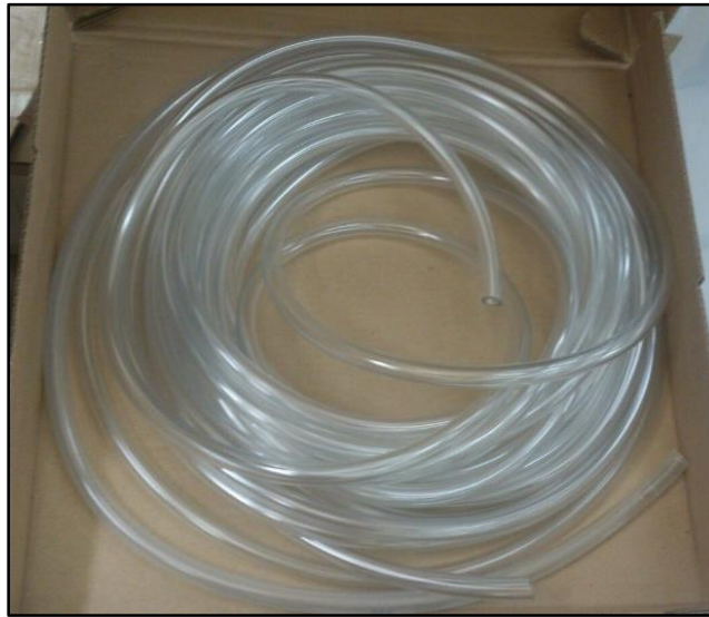
Figure 48: Vincon Feed and Permeate Tubing
