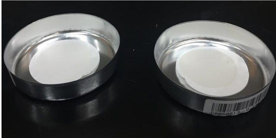
Figure 17: Drying filter paper used to calculate TSS
