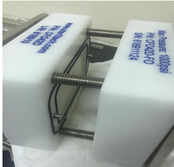
Figure 12: The two FO cell compartments. The left one is for the FS and the right one is for the DS separated by FO membrane which has a mesh spacer in feed side.
