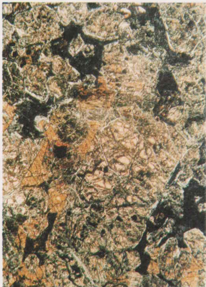
Fig. 2 : Mylonitized crystal lithic metatuff showing stretched quartz aggregates.
